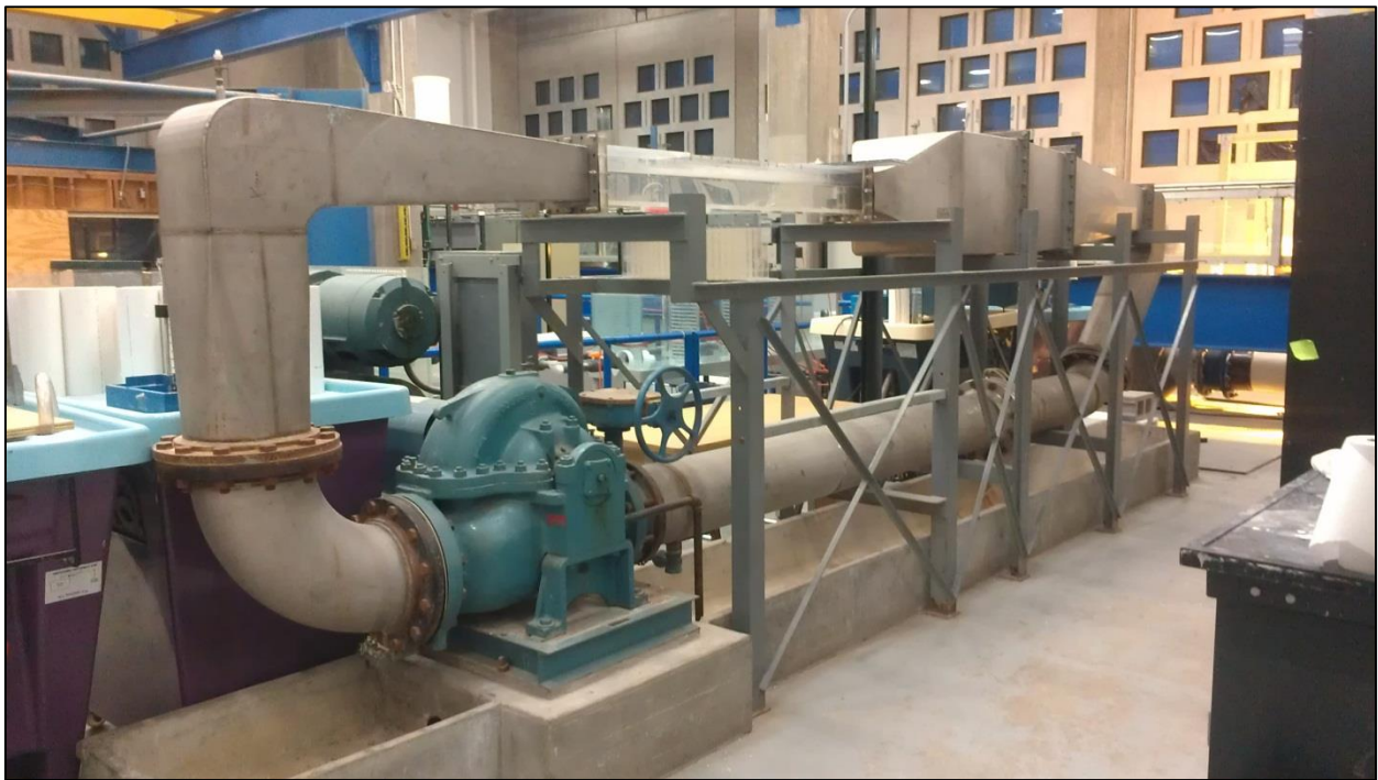
Figure 18: Recirculating flume apparatus used for creating ideal horizontal flow conditions.
